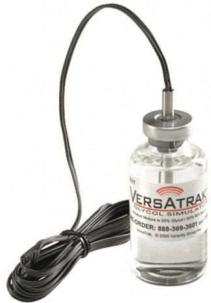
Buffered Temperature Probes are designed to prevent false readings by protecting the thermometer from sudden changes in temperature that can occur when opening a refrigerator door. A probe is "buffered" by immersing it in a vial filled with liquid (e.g., glycol, ethanol, glycerin), loose media (e.g., sand, glass beads), or a solid block of material (e.g. Teflon, aluminum)
